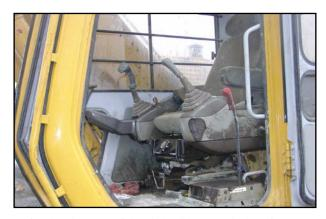
After leaning out of the right side cab window for a better view of the mechanic who was working near the bucket, the operator sat back down into his seat and his rain coat caught on the left-side control handle for the boom, causing the boom to swing and drop.
