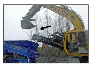
A mechanic was standing on the conveyor of a rock crusher (arrow), rigging the frame to an excavator bucket to lift the conveyor for maintenance. The excavator boom unexpectedly swung and dropped, and crushed him.
