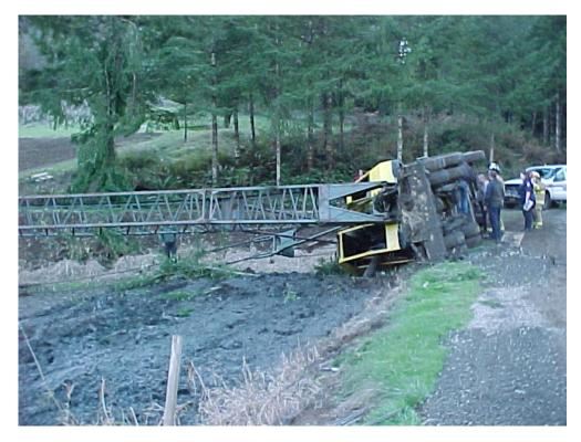
Photo 2. Crane topples over, crushing worker, while dredging dry fish pond. Note: outriggers were not deployed.
