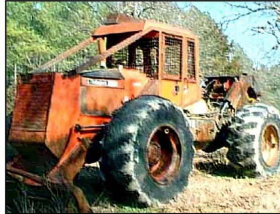
This stock photo of a skidder model like the one in this incident shows the step outside the cab where the operator was standing to hitch a ride.
