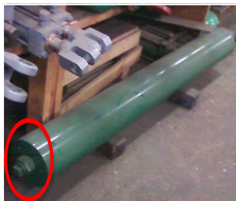
BELOW: Hydraulic accumulator (same model as in incident) with hydraulic pressure end cap shown in the red oval.
