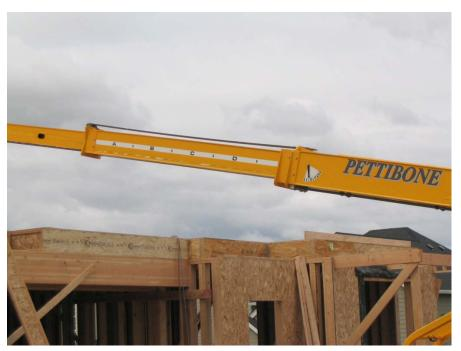
**Photo 4.** In upended position, the boom is extended between "D" and "E" load rating. Weight of load was calculated to be 3600-3800 lbs. extended ~24ft. The maximum load range at this reach and arc is 2000-3000 lbs.
