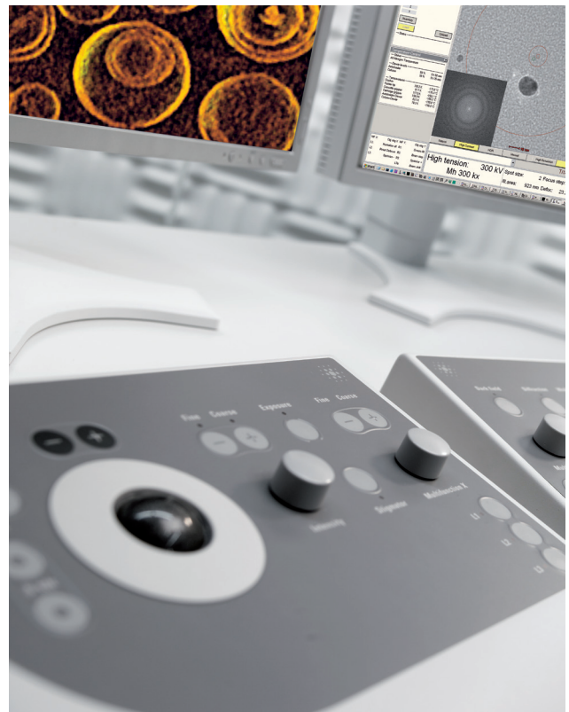
Figure 4: Primary control unit of the Titan Krios can be placed up to 15 meters from the microscope for ease of operation.
