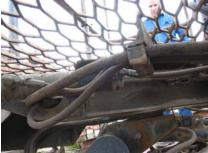
Fire investigators theorize that hot slag from the welding operation may have caused a pinhole size leak in the braided steel reinforced hose(s). It is also possible that other reasons exist for the failure of the hydraulic lines; e.g., defective hoses, overuse failure, age, and sudden catastrophic failure. The actual reason for hose
