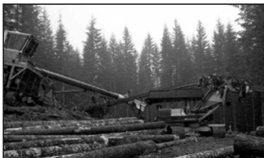
When guyline support failed, the yarder tower fell onto a nearby delimber (right).
