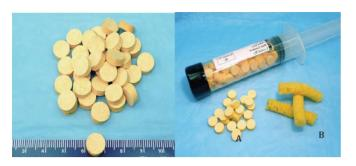
**Figure 1.** Prototype MSD and applicator. Note the degree of expansion between (*A*) dry MS and (*B*) wet MS.
