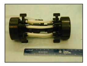
Figure 1: Elastin conduits mounted on curing manifolds
