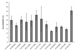
Figure 7 Percent water content of 13 batches of cured elastin conduits
