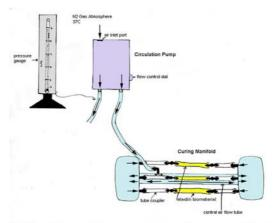
Figure 2: Diagram illustrating curing manifolds attached to circulation pump and pressure gauge with air-flow path indicated with black arrows
