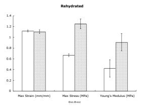
Figure 8 Ultimate strain, stress and Young's modulus data of cured EH1C (grey bar) and noncured EH1 elastin (white bar). Although the maximum strain remains unchanged, curing significantly increases the maximum stress and Young's modulus (p<0.01).
