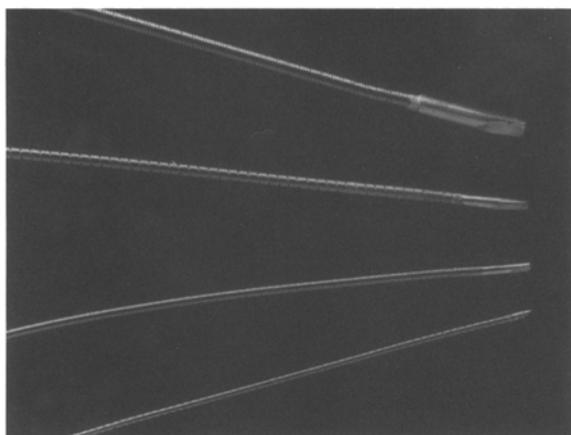
Fig. 9. Ultrasound transducers are getting smaller. Top-bottom; 0.088" for 9F, 12.5 MHz catheter, 0.054" for 6F, 20 MHz, 0.042" for 4.8F, 20 MHz, and 0.031AI for 3.5F, 30 MHz.
