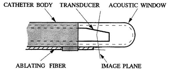
Fig. 1. Photo-acoustic catheter (PAAC) layout. Image plane intersects end of ablating fiber at side of acoustic window.
