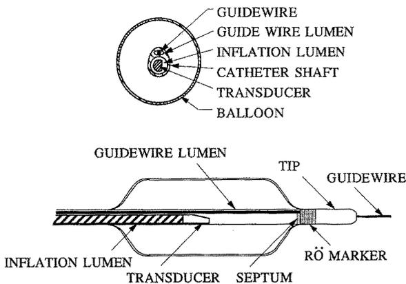
Fig. 6. Top: Cross-section of balloon ultrasound imaging catheter (BUIC). Transducer must image through catheter shaft and balloon material. Two-way attenuation through all layers is nearly 12 dB at 20 MHz. Bottom: Side view of BUIC. Transducer was positioned midway in all balloons used for clinical trials.
