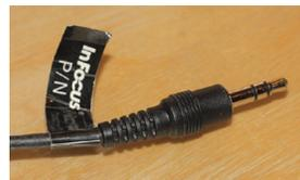
This 1/8" headphone-type cord will plug into most computers and provides sound capabilities when connecting with VGA.
