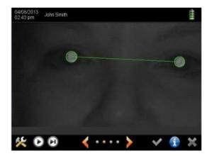
• When the distance is correct, the device will capture the image automatically along with a chime indicating its completion.
