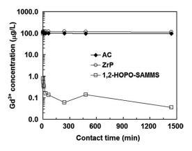
Figure 3. Adsorption kinetics of  $Gd^{3+}$  measured on 1,2-HOPO-SAMMS, activated carbon (AC), and zirconium phosphate (ZrP) in dialysate (pH 8.0), initial [Gd<sup>3+</sup>] of 100  $\mu$ g/L, L/S of 5000 mL/g.
