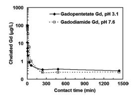
Figure 4. Adsorption kinetics of gadopentetate Gd and gadodiamide Gd measured on 1,2-HOPO-SAMMS, initial [chelated Gd] of 100  $\mu$ g/L, L/S of 5000 mL/g.
