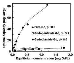
Figure 5. Adsorption isotherm of free Gd in dialysate (pH 8.0, L/S 100,000 mL/g), gadopentetate Gd in 0.1 M NaCl (pH 3.1, L/S 50,000 mL/g), and gadodiamide Gd in dialysate (pH 8.0, L/S 50,000 mL/g) measured on 1,2-HOPO-SAMMS.
