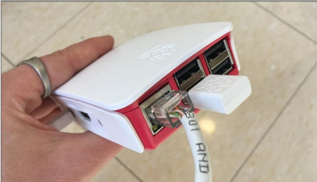
4. Connect the **Telegesis r310 dongle** to the hub computer, using one of the USB ports.
