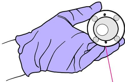
Four magnets for sampler removal
