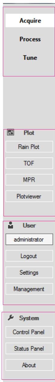
Acquire tab: Enables users to set up experiments (Experiment Manager), set acquisition limits and preview and record data.
