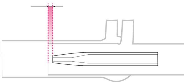
Figure 29. The injector should be positioned 1.5–2 mm from the end of the inner portion of the torch (as indicated by the pink dashed lines).
