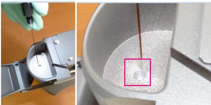
**NOTE** Handle this end of the sample probe line with care because it is used to acquire the sample.
