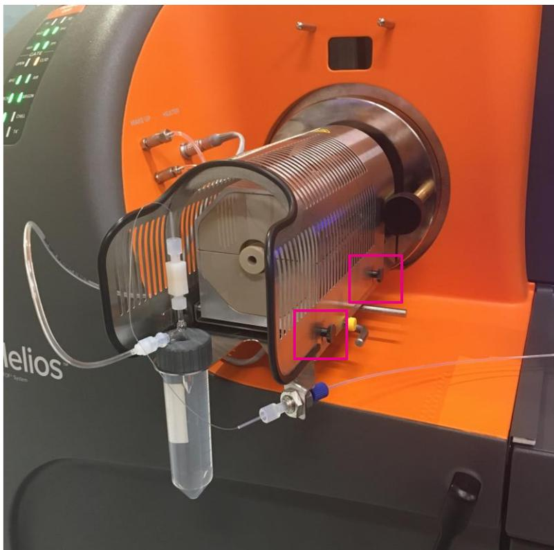
Figure 31. The heat shield on the Helios heater box. There are four screws, two on each side of the shield, that must be loosened before removing the shield.
