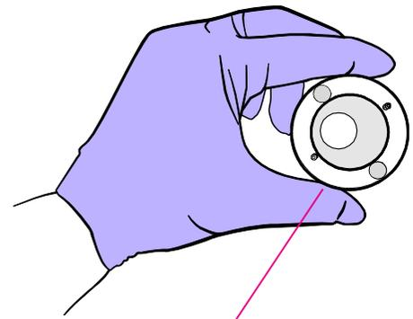
Two magnets for skimmer-reducer removal
