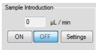
The Sample Introduction display indicates when the Sample Loader is on or off and shows the sample introduction flow rate. Users can click the **Settings** button to change the sample volumes.
