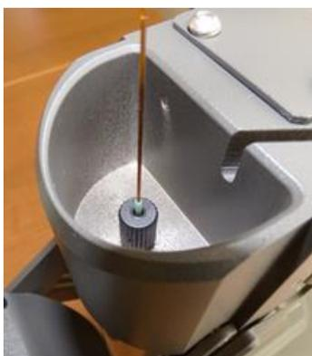
**NOTE** After tightening the black nut, if the green sleeve is loose, the Sample Loader will not pressurize. Loosen the black nut, remove all sample probe line parts, and repeat the procedure from step 5 (above).
