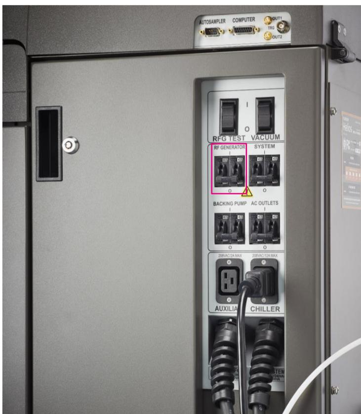
Figure 30. The RF generator circuit breaker on the Helios circuit breaker panel
