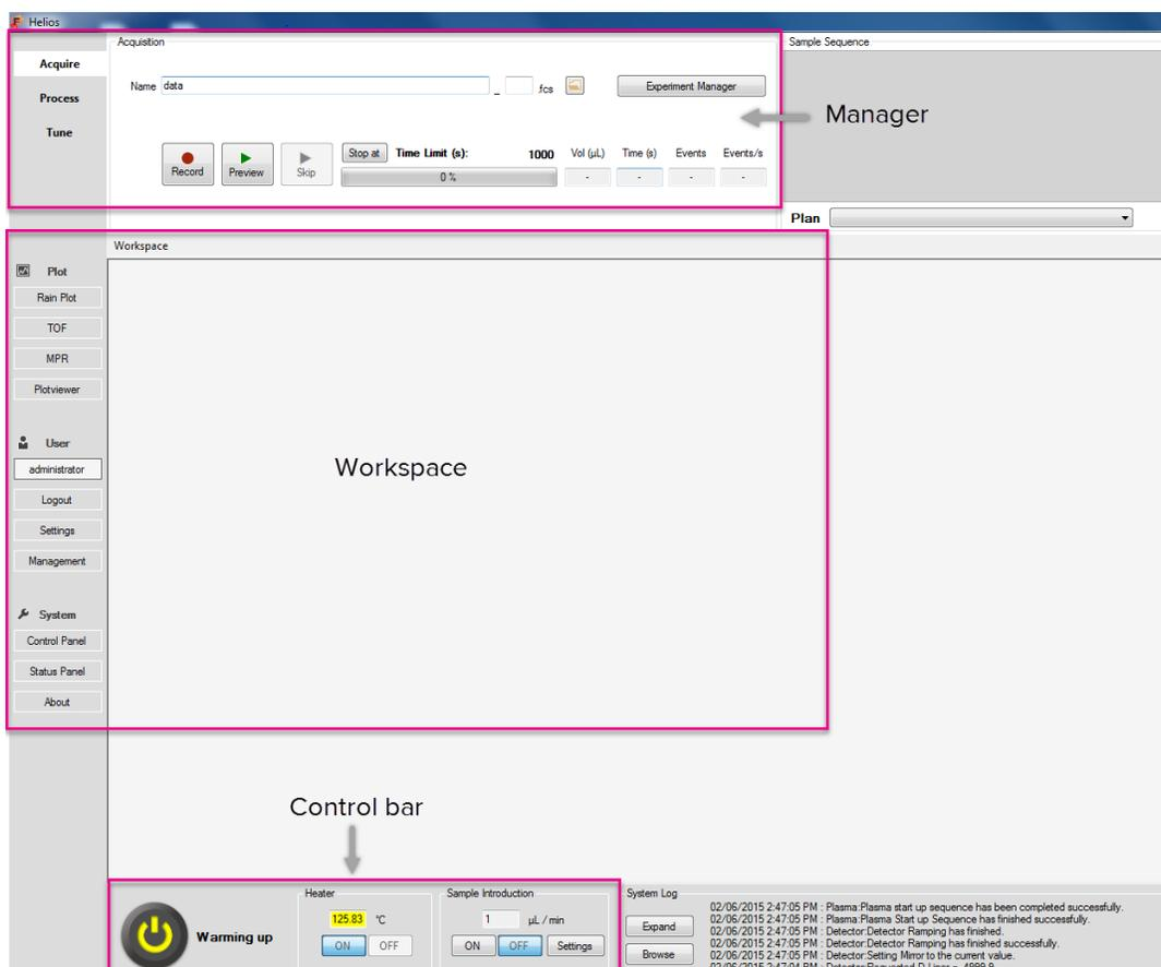
The Manager section, at the top of the start page, allows users to control sample volumes, set up tuning protocols, set up experiments, preview samples, acquire samples, and record results.
