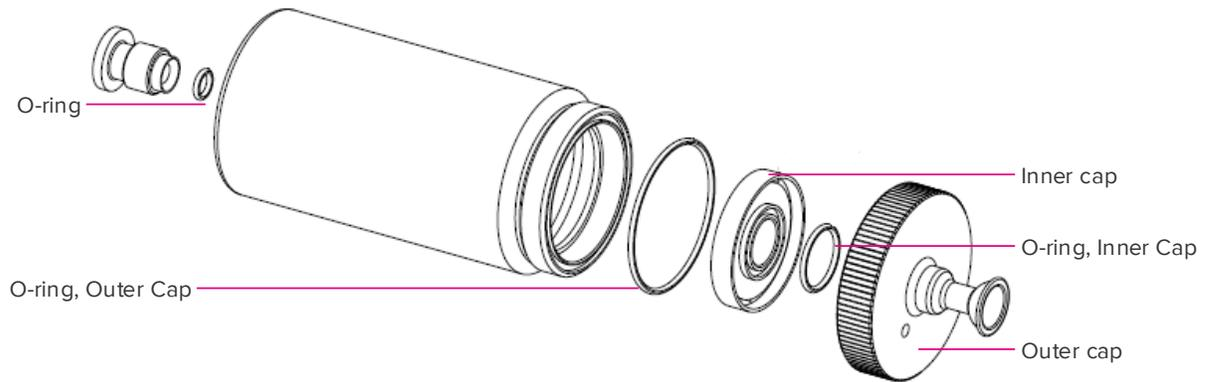
Figure 29. Spray chamber with outer cap and inner cap removed
