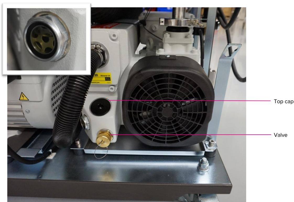
Figure 33. The interface pump in the lower right compartment of the Helios system. The visual inspection window is on the side of the interface pump (inset).
