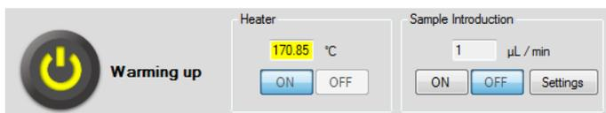
**NOTE** The plasma startup sequence will begin. The plasma, heater, and interface pump take approximately 15–30 minutes to warm up.
