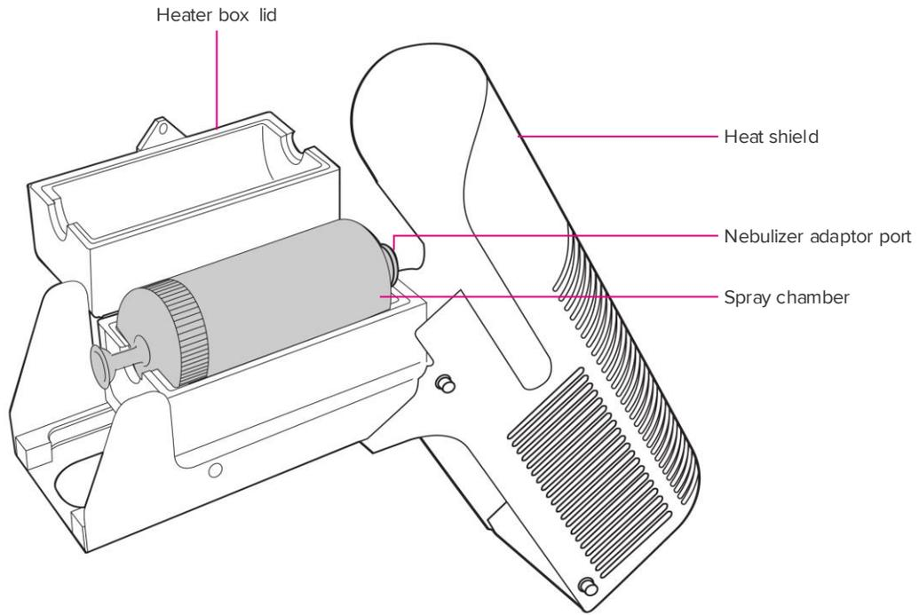
Figure 20. Spray chamber and connections
