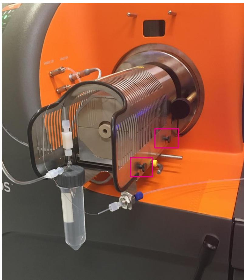
Figure 27. The heat shield on the Helios heater box. There are four screws, two on each side of the shield, that must be loosened before removing the shield.
