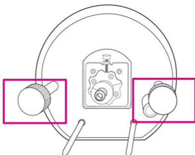
Figure 31. Torch assembly with thumbscrews (magenta boxes)
