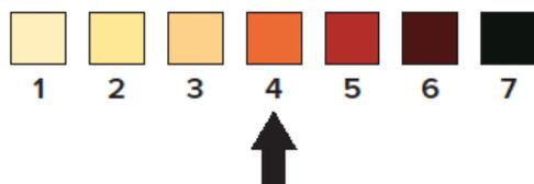
Figure 32. Pump oil condition chart. When the oil is above Level 4 (as indicated by the black arrow) the oil should be replaced in the interface pump.
