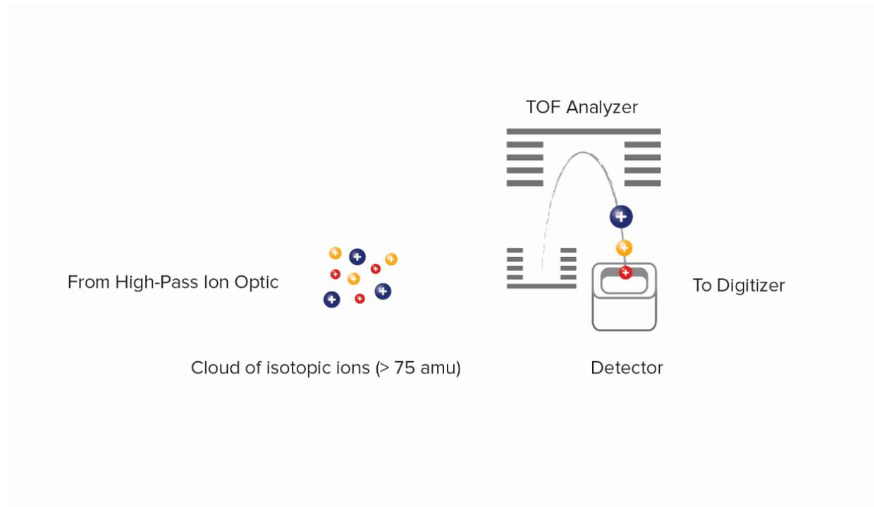
Figure 15. Separation of ions in the TOF. Ion clouds are subjected to an electrostatic force, which orthogonally accelerates the incoming ions toward the detector. As a result, the ions separate based on their mass-to-charge ratio, with lighter elements reaching the detector first.
