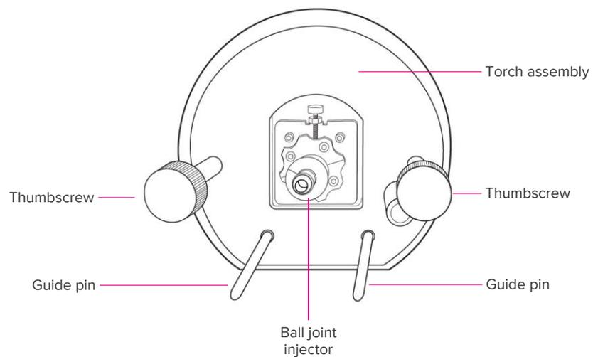
Figure 21. Front view of torch assembly
