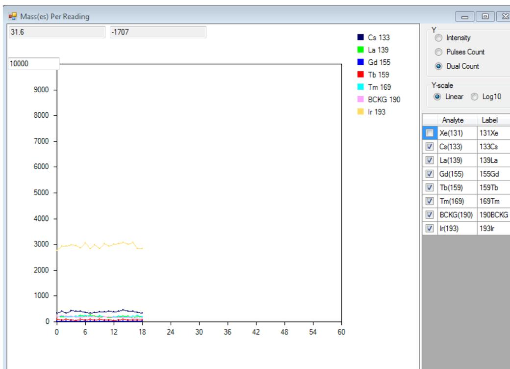
Figure 1. Masses per reading window. In this example, the 193Ir signal is very high which suggests the need for instrument maintenance (cleaning).
