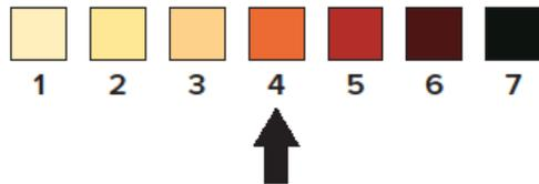
Figure 34. Pump oil condition chart. When the oil is above Level 4 (as indicated by the black arrow) the oil should be replaced in the interface pump.
