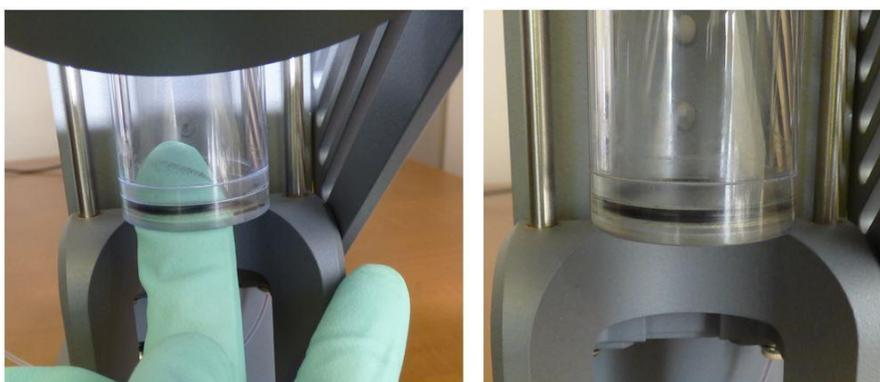
**NOTE** After replacing the O-ring, use a Kimwipes (as shown in step 3) to wipe any excess O-ring grease from inside the pressure chamber.
