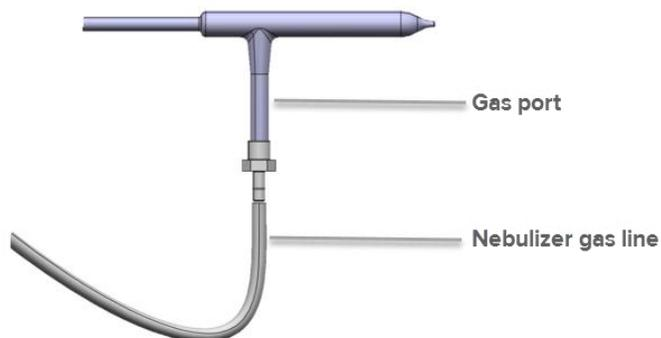
**NOTE** Check that the nebulizer gas line, the makeup gas line, and the heater quick-connects on the front of the instrument tightly fit.
