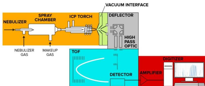
Figure 4. The Helios system. The mass cytometry workflow is divided into sample introduction and ionization (orange), ion transport through vacuum interface (green) high-pass ion optics (gray), ion separation in the time-of-flight (TOF) mass analyzer (blue), and data acquisition and processing (red).
